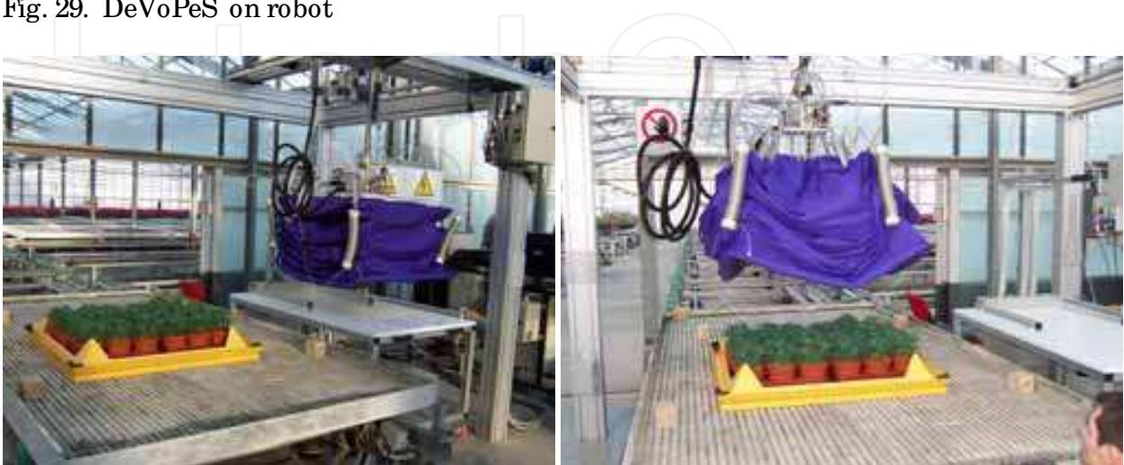
Fig. 30. DeVoPeS working in greenhouse
