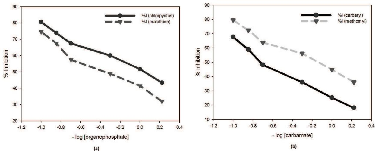
Fig. 5. Graphs of percentage inhibition vs.  $-\log$  [pesticide] results for two different organophosphorous pesticides in (a) and two different carbamate pesticides in (b). Results were obtained with the use of the Au/MBT/PANI/AChE/PVAc biosensor for six different pesticide concentrations evaluated.
