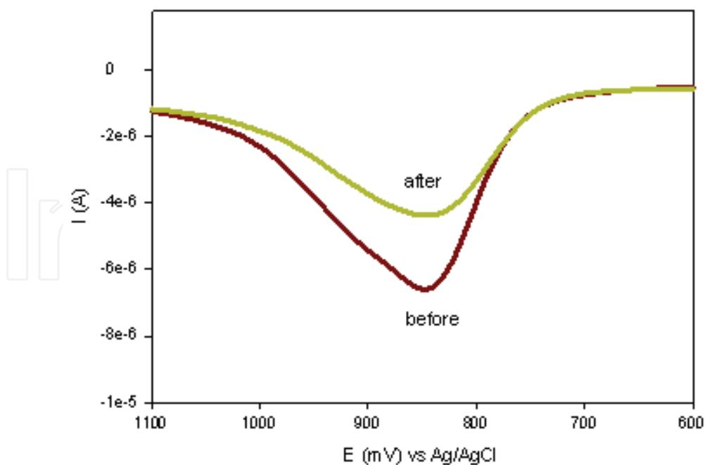
Fig. 3. Results for the DPV responses (before and after) of the Au/MBT/PANI/AChE/PVAc biosensor in a 0.1 M phosphate buffer, KCl (pH 7.2) solution in the presence of a 2 mM ATCh solution.
