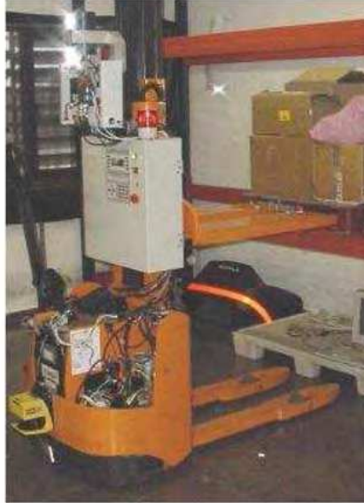
Fig. 5. Still EGV-10 robotized forklift used in a warehouse for realexperimentation. Odometry, laser positioning and monocular vision data were recollected.
