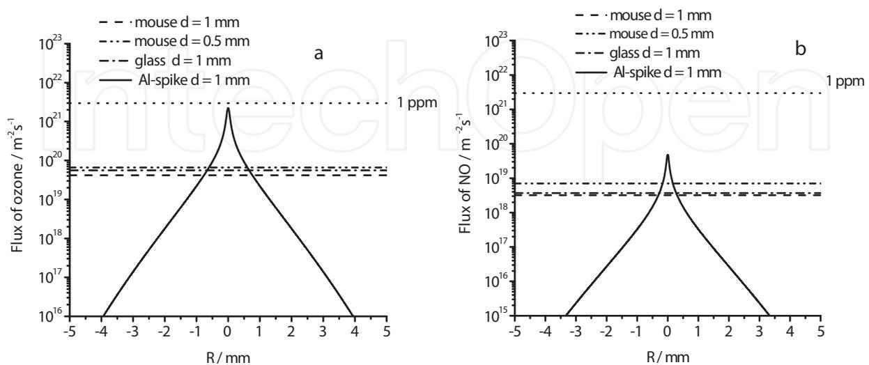
Fig. 10. Flux of ozone (a) and nitric oxide (b) reaching the treated surface across the radius of the driving electrode ( $R$ ) for DBD on different substrates. The fluxes at species' concentration of 1 ppm are calculated using mean velocity and concentration of nitrogen and oxygen molecules at plasma conditions.
