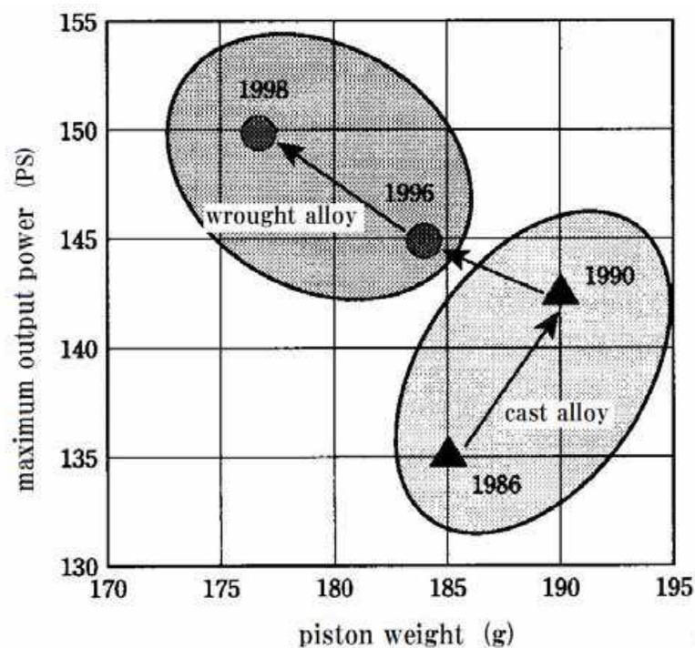
Fig. 6. Historical review of the relation between maximum output power and aluminum alloy piston weight for 1,000cm<sup>3</sup> engine<sup>35)</sup>
