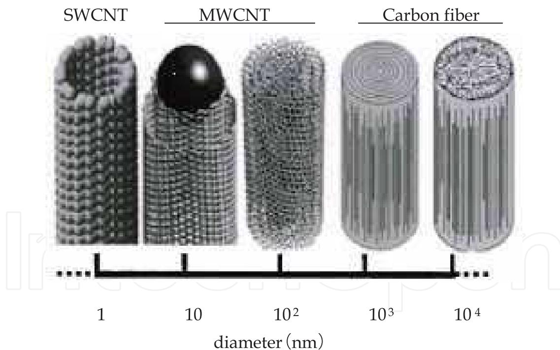
Fig. 1. Illustration sorting carbon fiber and CNTs<sup>24)</sup>
