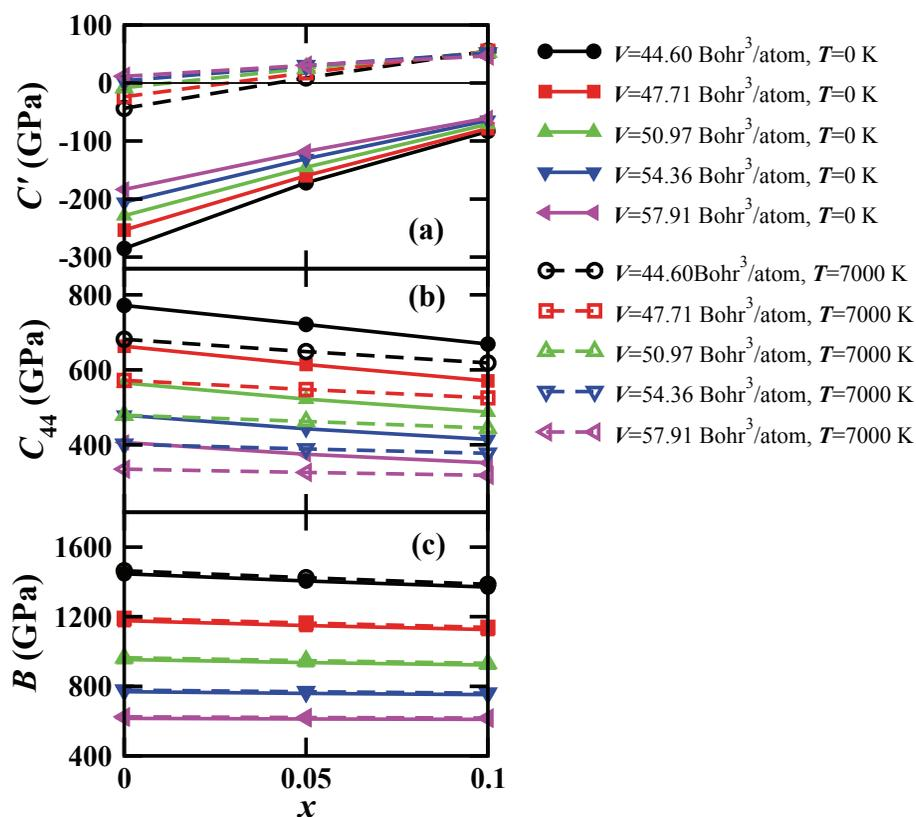
Fig. 8. Single crystal elastic constants,  $C'$ ,  $C_{44}$ , and the bulk modulus,  $B$ , as a function of Mg concentration,  $x$ , calculated at different  $V$  volumes at zero temperature (solid lines) and at  $T=7000$  K (dashed lines). The horizontal black line in panel (a) corresponds to  $C'=0$  GPa.
