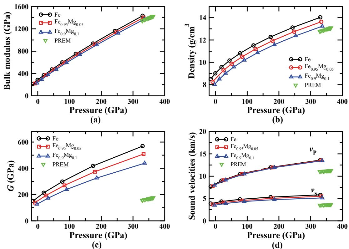
Fig. 6. Theoretical bulk modulus (a), density (b), shear modulus,  $G$  (c), and sound velocities (d) of pure hcp Fe (circles),  $\text{Fe}_{0.95}\text{Mg}_{0.05}$  (squares) and  $\text{Fe}_{0.9}\text{Mg}_{0.1}$  (triangles) as a function of pressure.  $v_p$  and  $v_s$  denote longitudinal and transverse sound velocities, respectively. Seismic data as given in the PREM model are shown for comparison (inverted triangles).
