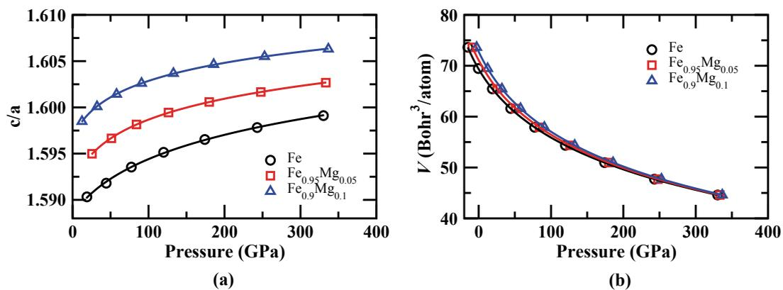
Fig. 5. Theoretical pressure dependency of the hexagonal axial ratios ( $c/a$ ) and the volume of pure hcp Fe (circles),  $\text{Fe}_{0.95}\text{Mg}_{0.05}$  (squares) and  $\text{Fe}_{0.9}\text{Mg}_{0.1}$  (triangles).
