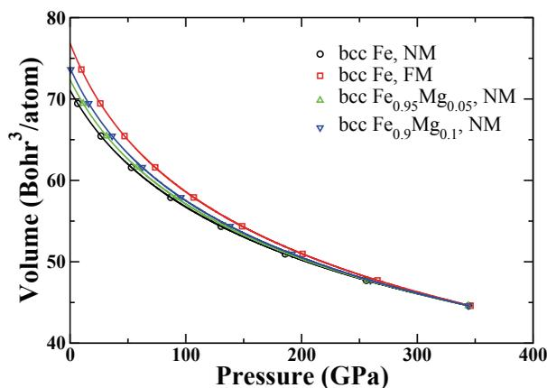
Fig. 7. Calculated equation of state for nonmagnetic (NM) and ferromagnetic (FM) pure bcc Fe (denoted by black circles and red squares, respectively), NM bcc  $\text{Fe}_{0.95}\text{Mg}_{0.05}$  (red triangles), and bcc  $\text{Fe}_{0.9}\text{Mg}_{0.1}$  alloys (blue inverted triangles).
