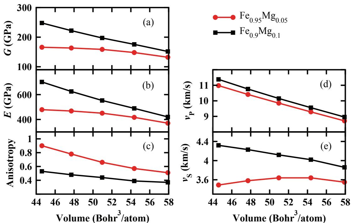
Fig. 10. Shear ( $G$ ) and Young moduli ( $E$ ), polycrystalline anisotropy, and longitudinal ( $v_P$ ) and transversal ( $v_S$ ) sound velocities of bcc Fe<sub>0.95</sub>Mg<sub>0.05</sub> (red circles) and Fe<sub>0.9</sub>Mg<sub>0.1</sub> alloys (black squares) at different  $V$  volumes, at  $T=7000$  K temperature.
