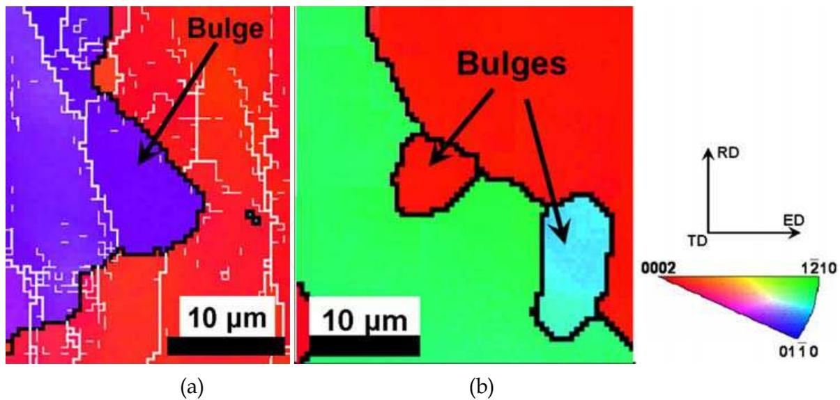
Fig. 14. Inverse pole figure (IPF) maps of an AM30 sample deformed to 0.2 strain; three examples of bulge nucleation are shown. The low-angle boundaries ( $2^\circ < \omega < 15^\circ$ ) are shown in white and the high-angle boundaries ( $\omega \geq 15^\circ$ ) in black. The IPF color triangle indicates the orientation of the TD axis in the hexagonal crystal reference system.
