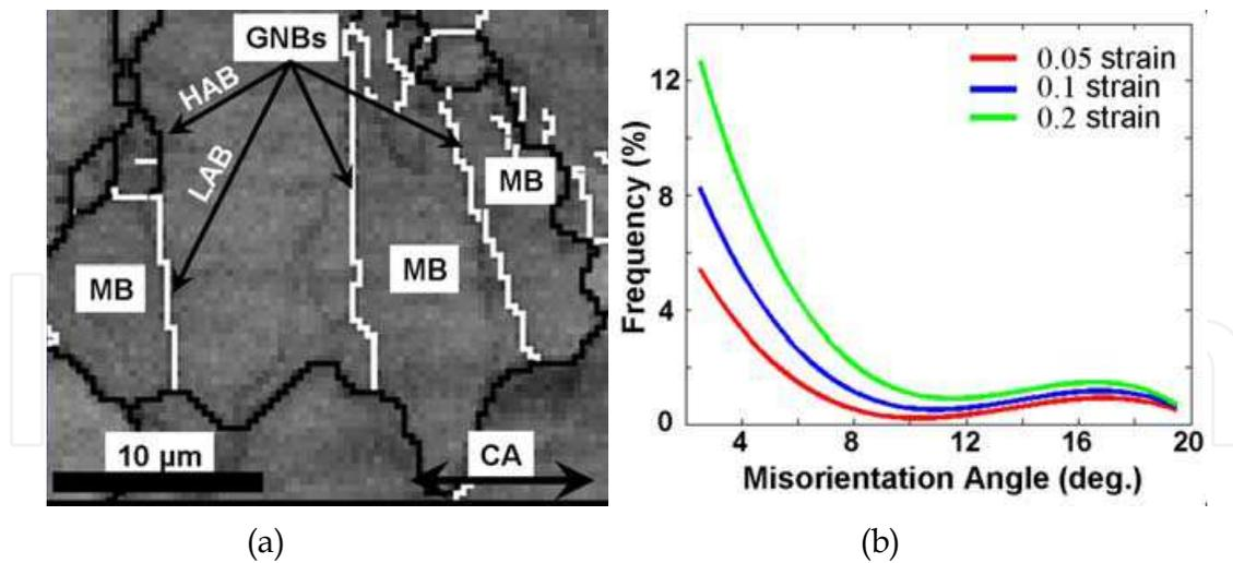
Fig. 9. (a) EBSD map illustrating the geometrically necessary boundaries (highlighted by the black arrows) that delineate microbands. The low-angle boundaries ( $5^\circ < \omega < 15^\circ$ ) are shown in white and the high-angle boundaries ( $\omega \geq 15^\circ$ ) in black. (b) Misorientation frequencies of the boundaries developed during the hot compression of magnesium AM30.
