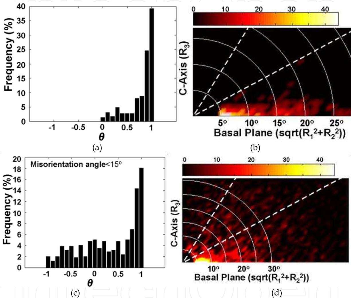
Fig. 12. c-axis displacements towards the CA direction attributable to the formation of (a) microbands and kinkbands and (c) subgrains. Side views of the reduced zones<sup>3</sup> displaying the rotations associated with (b) MBs and KBs and (d) new grains. The two dashed white lines represent vectors that are inclined at 30° and 60° to the c-axis and the white quarter circles identify the misorientation angles associated with the Rodrigues-Frank (RF) vectors.
