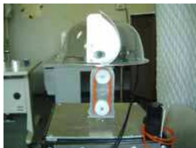
Figure 4. Side view of the robot with pinnae
