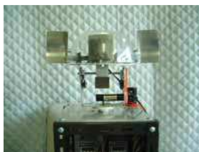
Figure 3. Front view of the robot with pinnae
