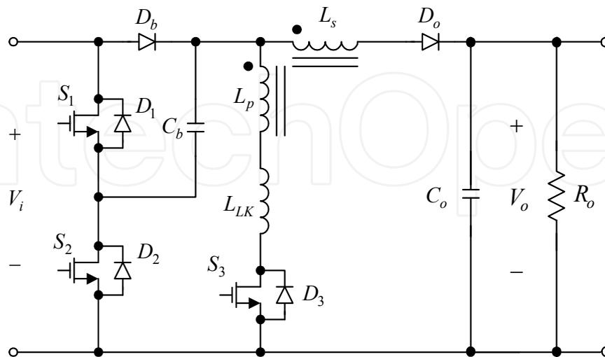
Fig. 2. Proposed voltage-boosting converter with leakage inductance considered.
