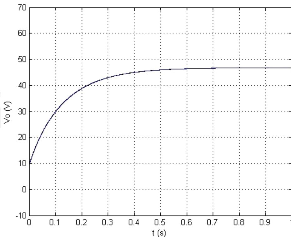
Fig. 14. Simulated output voltage during startup.
