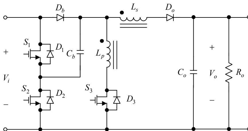
Fig. 1. Proposed voltage-boosting converter without leakage inductance considered.
