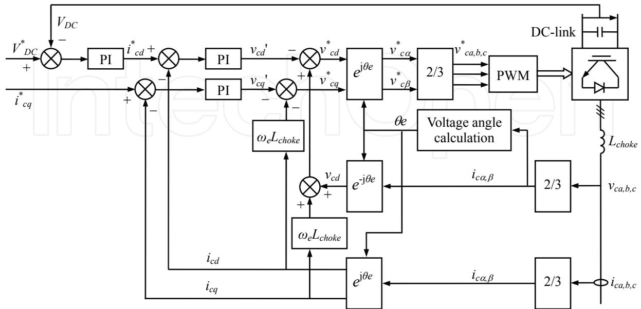
Fig. 12. Vector control structure for grid-side converter.
