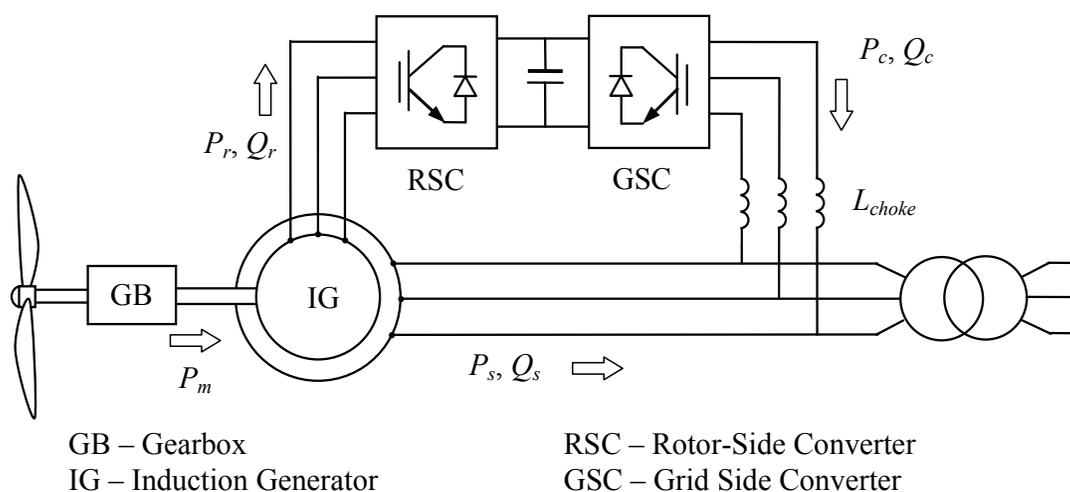
Fig. 8. Doubly-fed induction generation system power flows.
