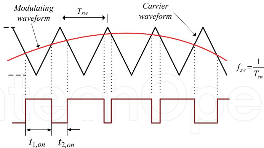
Fig. 7. Example of carrier-based pulse-width modulated signal generation.
