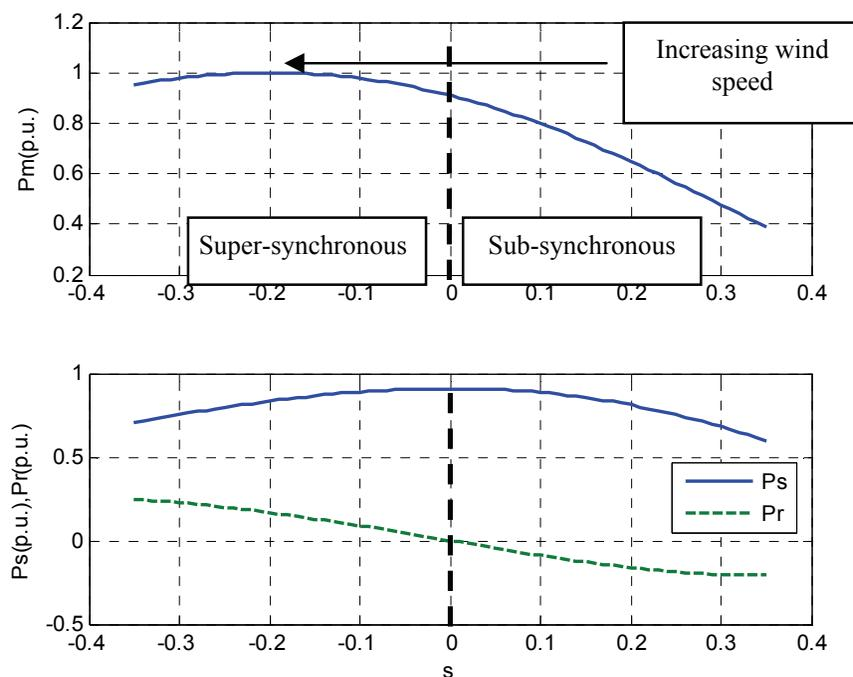
Fig. 9. Doubly-fed induction generation system power flows.
