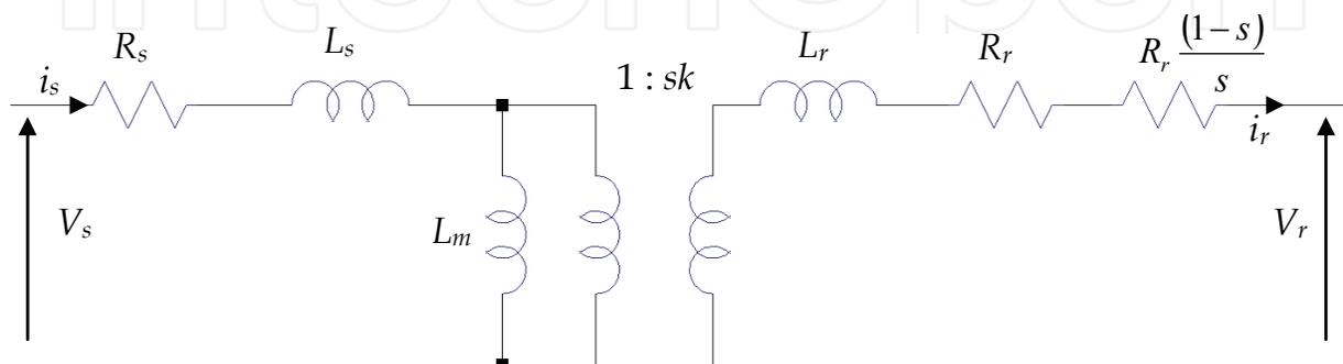
Fig. 2. Per-phase equivalent circuit of an induction machine.
