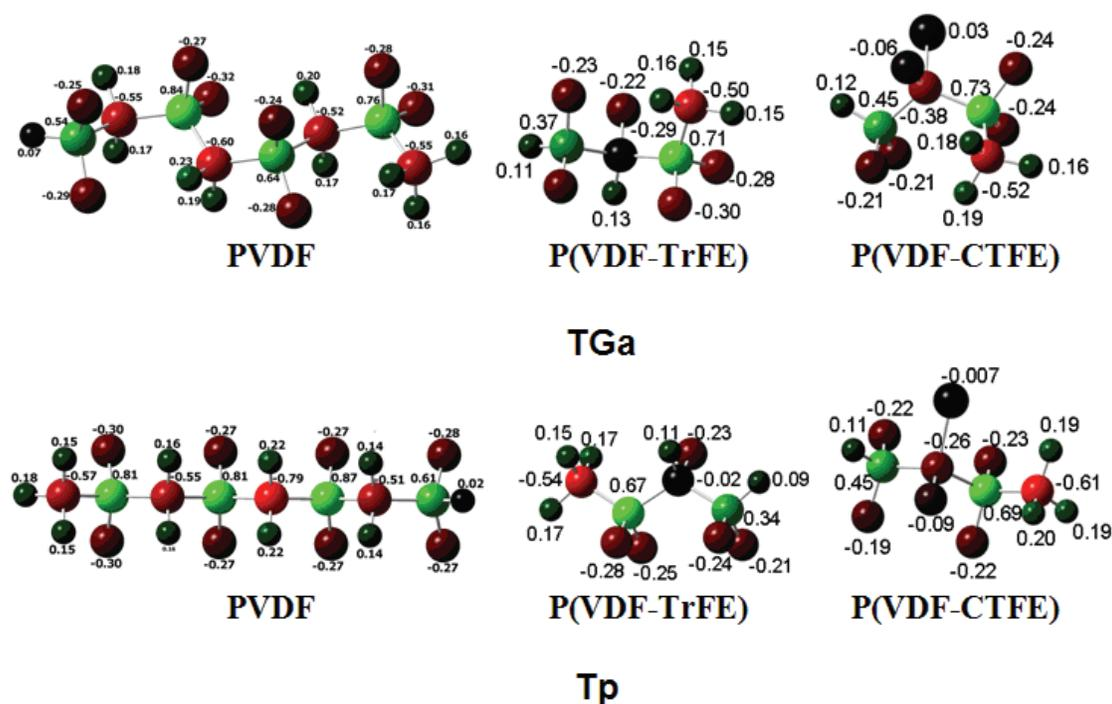
Fig. 7. ESP charge representation for  $TG_a$  and  $T_p$  of the representative model of the different materials, namely, PVDF, P(VDF-TrFE) and P(VDF-CTFE). Negative charge values are in red, positive charge values are in dark green and the larger positive charges are depicted in light green.
