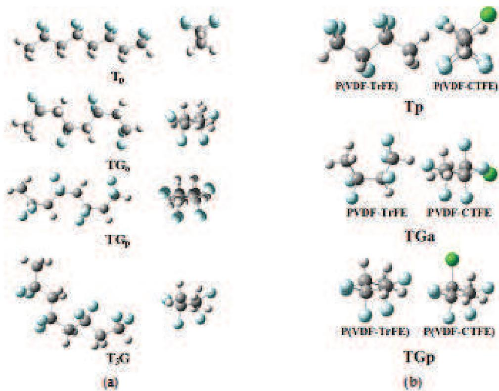
Fig. 1. Structural representation for the different PVDF conformers, namely,  $T_p$ ,  $TG_a$ ,  $TG_p$  and  $T_3G$ . Fluorine atoms are in blue, carbon atoms are in grey and hydrogen atoms are in white. a) PVDF b) P(VDF-TrFE) and P(VDF-CTFE).
