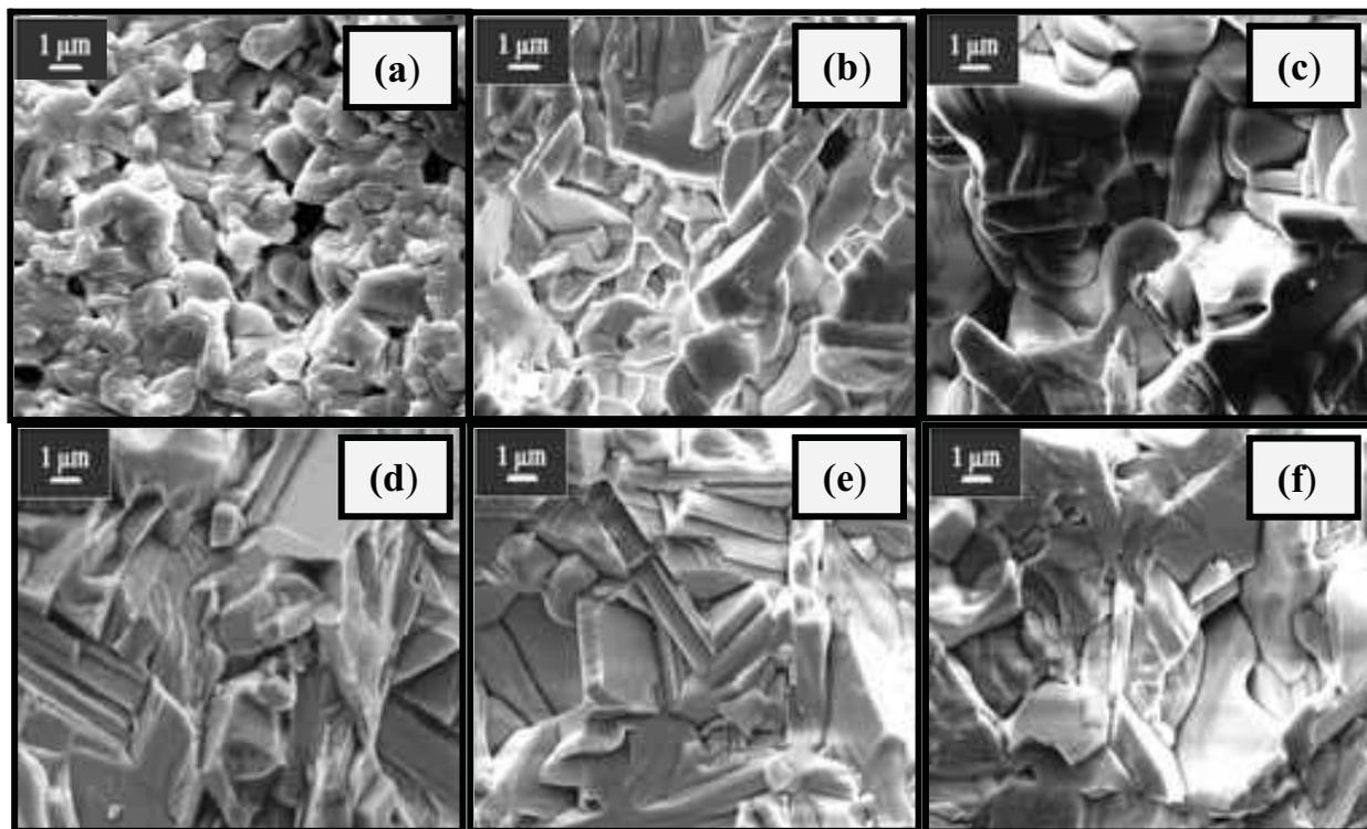
Fig. 3. SEM images with (a)  $x = 0.0$ , (b)  $x = 0.025$ , (c)  $x = 0.05$ , (d)  $x = 0.075$ , (e)  $x = 0.10$  and (f)  $x = 0.20$  of  $\text{SrBi}_2(\text{Ta}_{1-x}\text{W}_x)_2\text{O}_9$  samples
