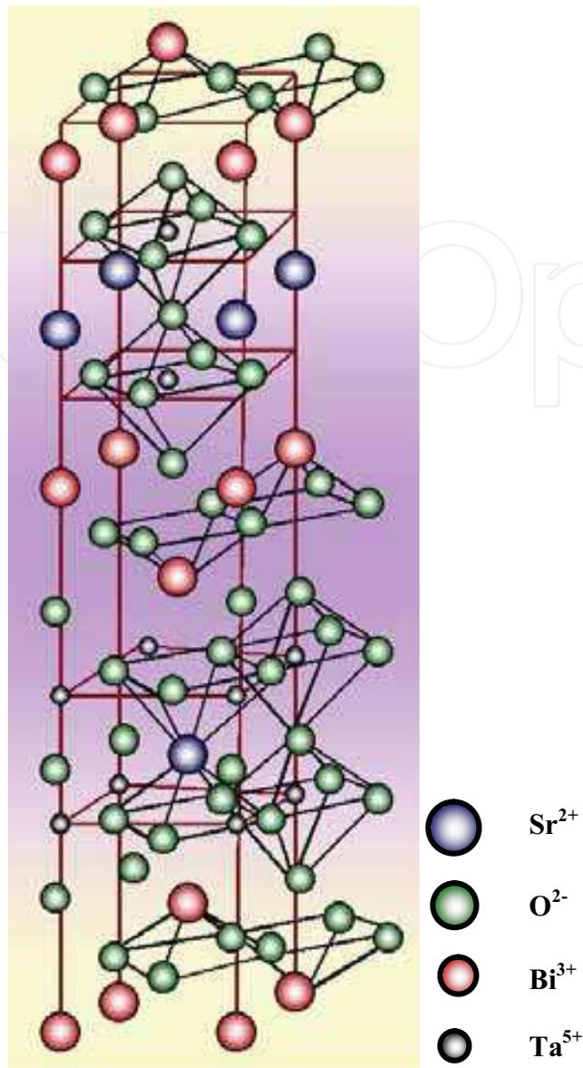
Fig. 1. The crystal structure of SrBi<sub>2</sub>Ta<sub>2</sub>O<sub>9</sub>
