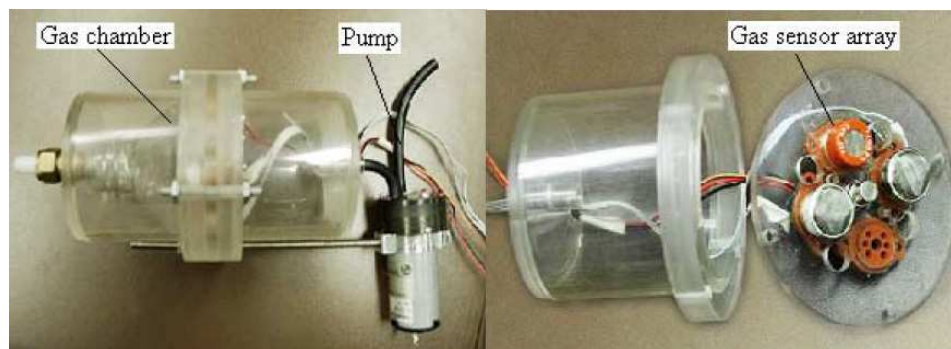
Fig. 5. E-nose with gas chamber, pump and sensor array exerted from (Jianfeng et al. , 2009)
