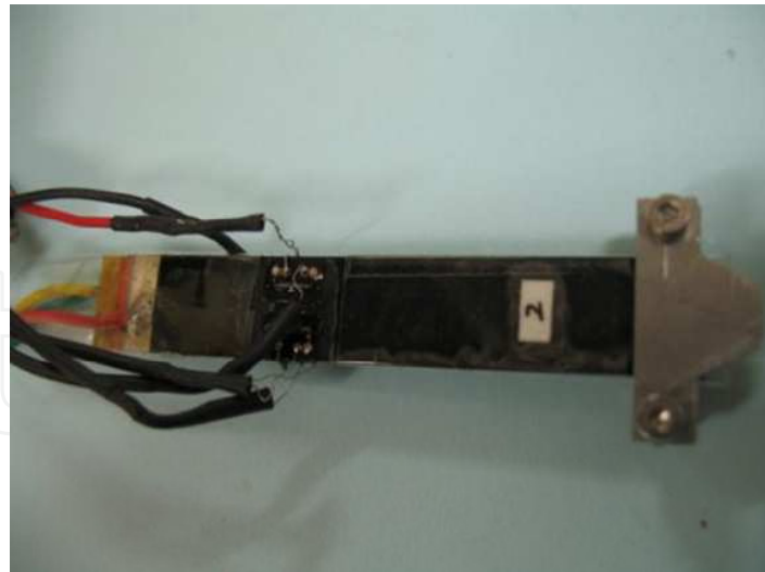
Fig. 9. Macle piezoelectric ceramics affixed with strain gages
