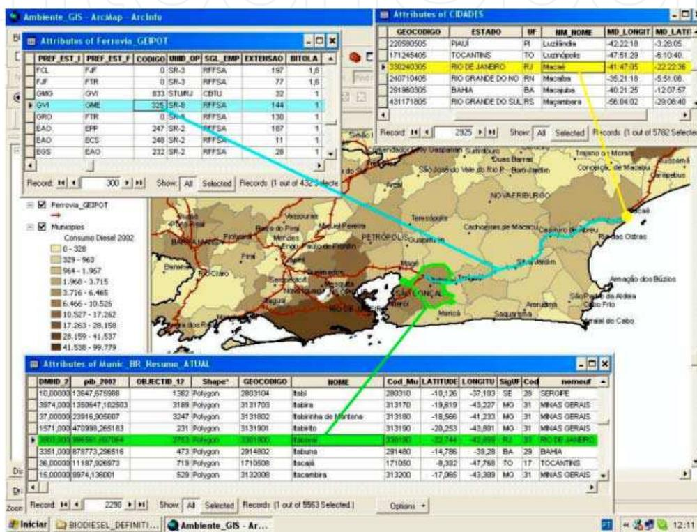
Fig. 8. Vector features as point, line and polygon with associated table containing geocode
