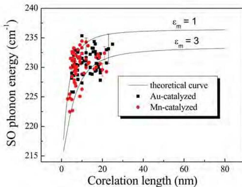
Fig. 14. Comparison of experimental and theoretical results for SO phonon vs correlation length. Solid line indicates the curve calculated by using the model presented by Ruppin *et al.* [49] for two different values of the dielectric constant of the surrounding medium. Experimental data points for Mn-catalyzed InAs NWs (dots) and Au-catalyzed InAs NWs (squares) located on the theoretically calculated curve for the SO phonons in terms of correlation length
