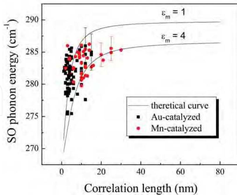
Fig. 13. Comparison of experimental and theoretical results for SO phonon vs correlation length. Solid line indicates the curve calculated by using the model presented by Ruppin *et al.* [49] for two different values of the dielectric constant of the surrounding medium. Experimental data points for Mn-catalyzed GaAs NWs (dots) and Au-catalyzed GaAs NWs (squares) located on the theoretically calculated curve for the SO phonons in terms of correlation length
