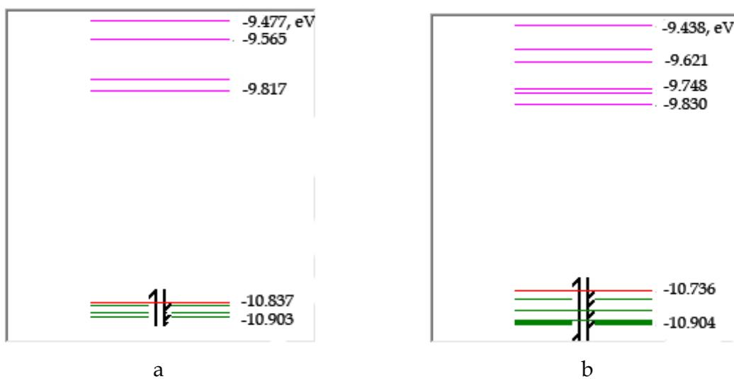
Fig. 18. The energy-band structure of the base nanotube with indices (6,5) after passivation the dangling bonds by atoms of hydrogen: (a) - 200-atomic model; (b) - 400-atomic model.
