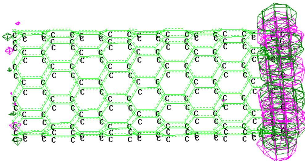
Fig. 3. Orbital 413 of the carbon nanotube with indices (10,0).
