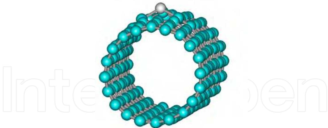
Fig. 10. Optimised geometry of the Al-doped carbon (10,0) nanotube.
