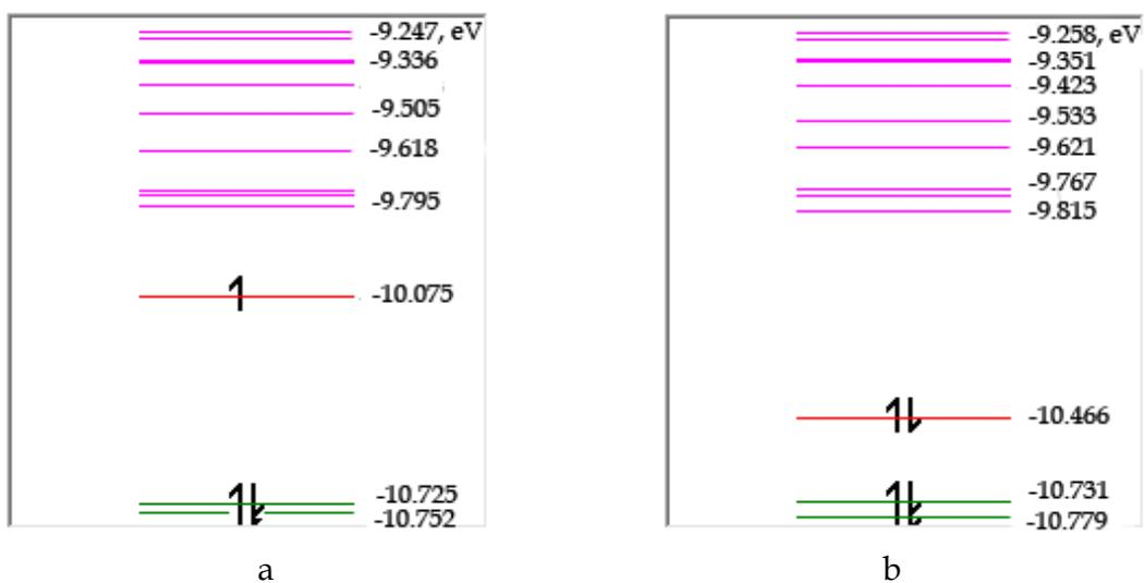
Fig. 32. The phosphorus-doped 410-atomic carbon (6,5) nanotube: (a) - hydrogen endings on edges of a nanostructure; (b) - the complete hydrogen endings.
