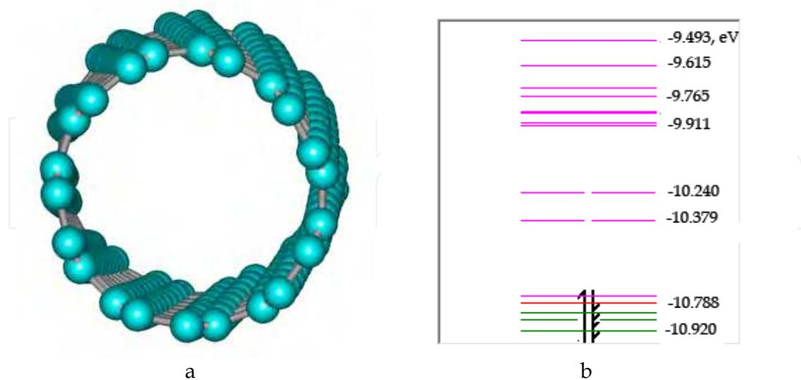
Fig. 16. 200-atoms basic model (a) and energy-band structure (b) of a carbon nanotube with indices (6,5).
