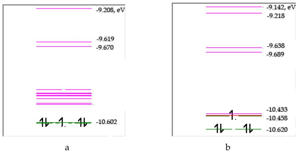
Fig. 9. Effect of impurity atom of nitrogen on energy spectrum of the carbon (10,0) nanotube before (a) and after (b) hydrogen ending.
