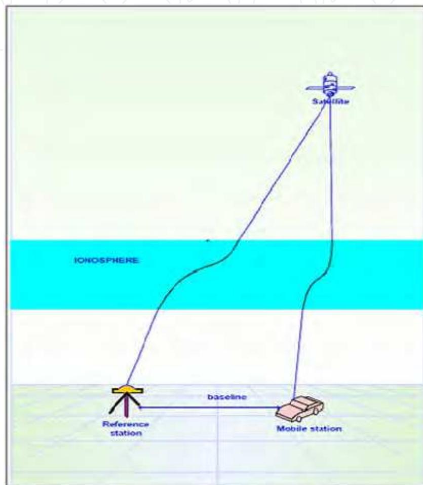
Fig. 1. Exaggerated view of GPS signal geometric paths
