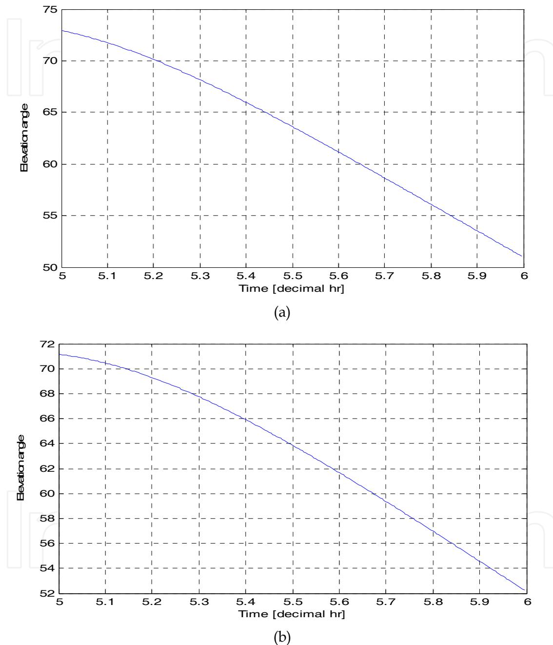
Fig. 7. (a) Elevation angle of GPS Satellite PRN 23, 5:00-6:00 (UT) (KTPK station)
