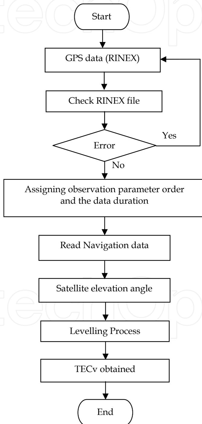
Fig. 3. Flowchart of TEC processing
