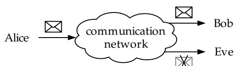
Fig. 1. Communication system with a transmitter (Alice), a legitimate receiver (Bob) and an eavesdropper (Eve).
