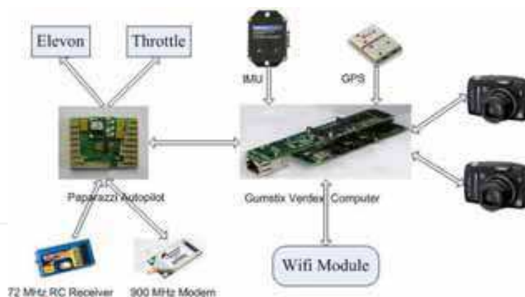
Fig. 8. AggieAir Airborne System Structure.
