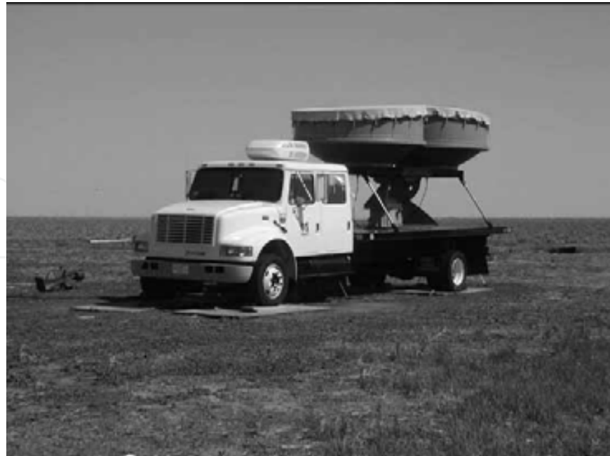
Fig. 3. The University of Massachusetts S-Band FMCW radar system mounted on flatbed truck (electronics are contained within the cab).
