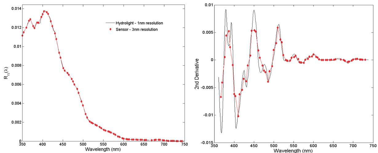
Fig. 11. (Left) An example of a simulated hyperspectral remote-sensing reflectance,  $R_{rs}(\lambda)$ , before and after applying the modeled sensor's response (black and red curves, respectively). (Right) Second derivatives of spectra in the left panel.
