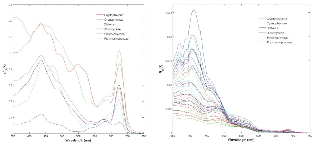
Fig. 9. (Left) Specific absorption spectra of six phytoplankton groups. (Right) Simulated hyperspectral  $R_{rs}(\lambda)$  spectra (1 nm resolution) corresponding to different dominating phytoplankton groups at different concentrations (0.01, 0.03, 0.05, 0.07 and 0.09  $\text{mg}/\text{m}^3$ ).
