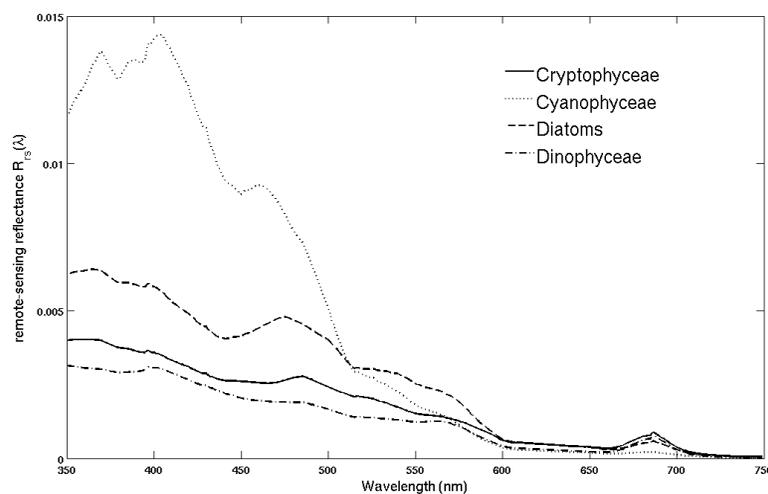
Fig. 7. Results of Hydrolight radiative transfer simulations, showing four remote-sensing reflectances  $R_{rs}(\lambda)$  (1 nm resolution) obtained under different composition conditions. Labels indicate each dominant phytoplankton group considered in each case.
