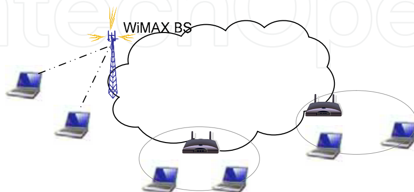
Fig. 7. Integrated WiMAX/WiFi wireless access.
