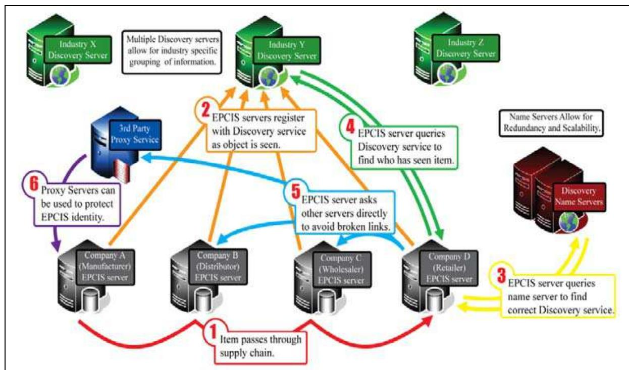
Fig. 5. EPCglobal network architecture (Beier *et al.*, 2006)
