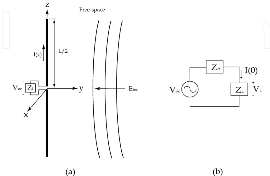
Fig. 3. (a) A thin-wire dipole in free-space; (b) the equivalent circuit of the receiving dipole. Next, consider the equivalent circuit of the receiving dipole shown in Fig. 3 (b) where  $Z_L$  and  $Z_A$  are the load and antenna impedance values, respectively. Using voltage division, the load voltage can be written as
