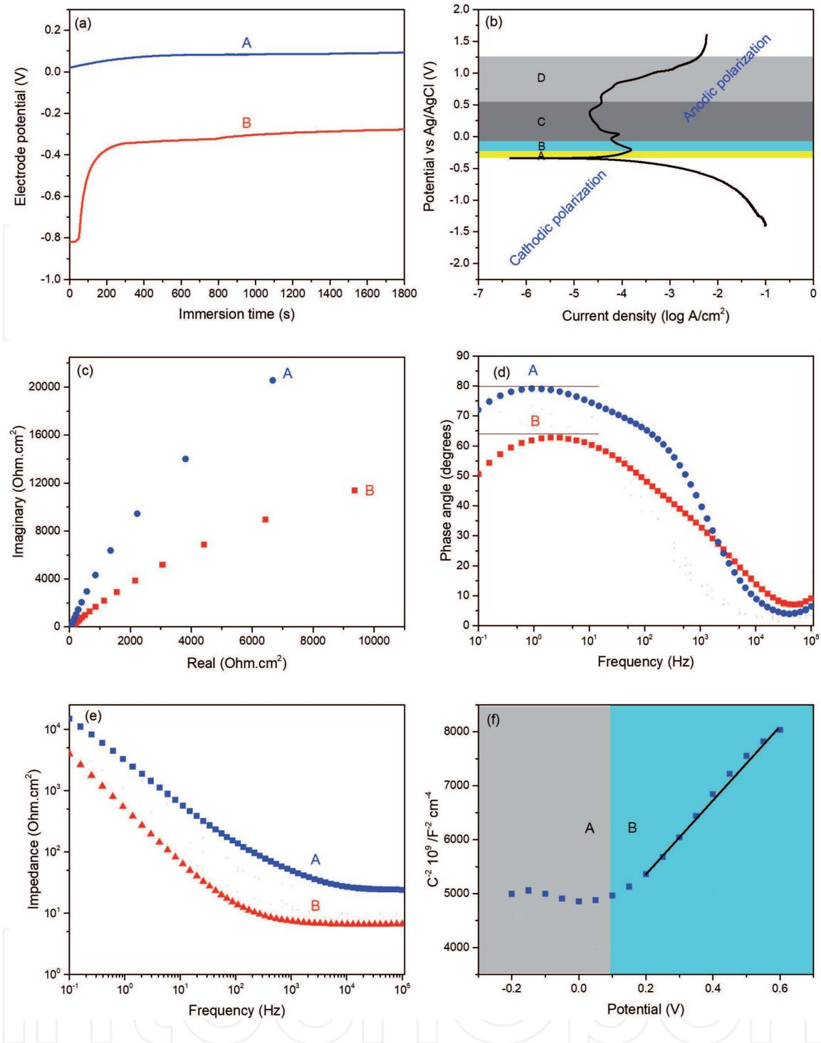
**Figure 1.** Illustration of the corrosion properties of metallic materials; (a) open circuit potential (OCP), (b) potentiodynamic polarization, (c) Nyquist plot, (d) Bode phase angle plot, (e) Bode impedance plot, and (f) Mott-Schottky plot.
