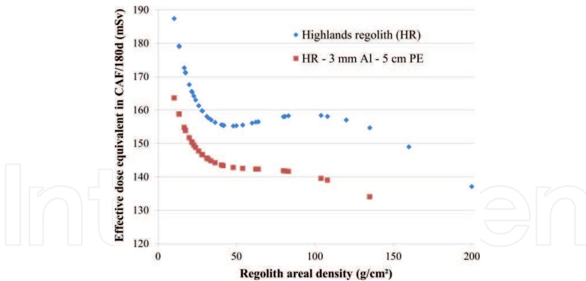
**Figure 2.** Effective dose equivalent from GCR in CAF/180 days behind highlands regolith (HR) and multilayer shielding (HR—3 mm aluminum, Al—5 cm polyethylene, PE) as a function of regolith areal density. Based on results in [39].
