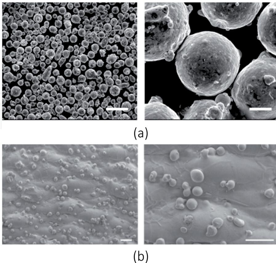
**Figure 6.** FESEM images. (a) Cobalt chromium alloy powder in size range of 25–40  $\mu\text{m}$ . Scale bars are 100  $\mu\text{m}$  (left) and 10  $\mu\text{m}$  (right). (b) Surface of a part made by sintering of cobalt-chromium alloy. Scale bars are 100  $\mu\text{m}$ .
