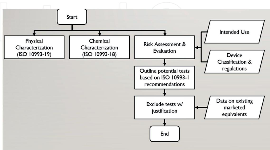
**Figure 11.** Flowchart of selection of biocompatibility tests.
