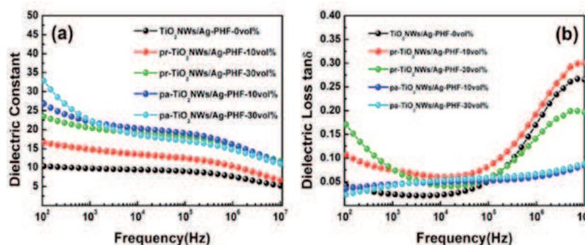
**Figure 3.** Frequency dependence of (a) dielectric constant and (b) dielectric loss ( $\tan \delta$ ) of Ag-TiO<sub>2</sub>-P(VDF-HFP) ternary composites. Reprinted with permission from ref. [78].
