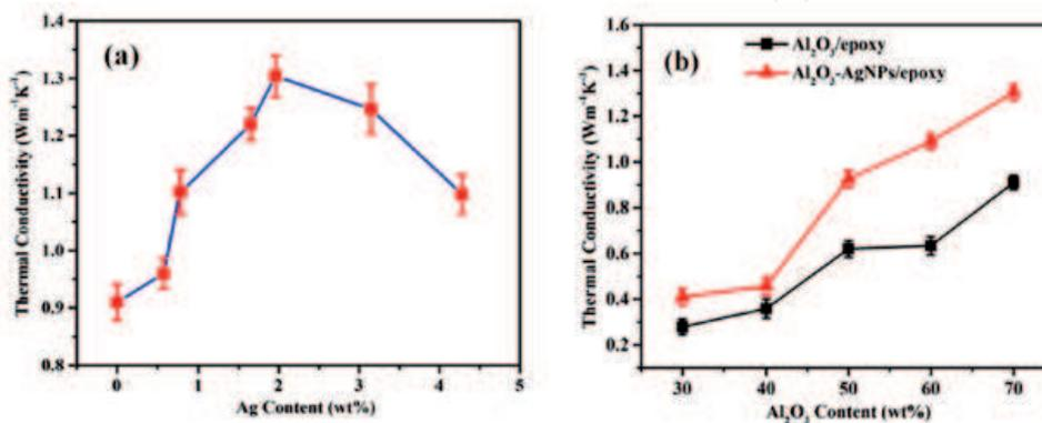
**Figure 2.** Thermal conductivity of (a)  $\text{Al}_2\text{O}_3\text{-Ag NPs-epoxy}$  composites as a function of Ag contents, (b) variation of thermal conductivity of  $\text{Al}_2\text{O}_3\text{-epoxy}$  and  $\text{Al}_2\text{O}_3\text{-AgNP-epoxy}$  composites. Reprinted with permission from ref. [64].
