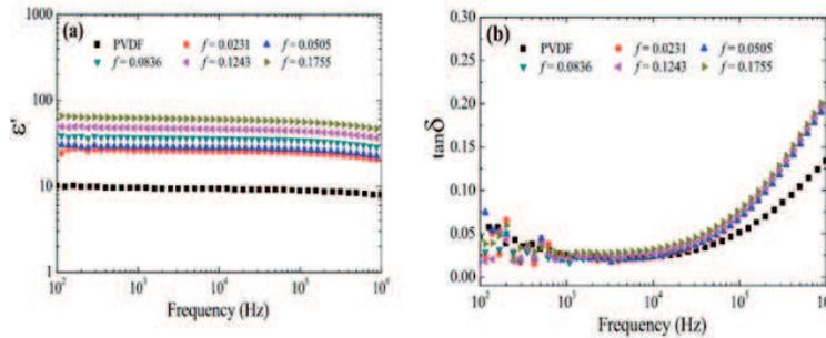
**Figure 1.** Frequency dependence of (a) dielectric permittivity ( $\epsilon'$ ) and (b) dielectric loss ( $\tan \delta$ ) of  $n\text{Ag-MLSNO-PVDF}$  composites. Reprinted with permission from ref. [63].
