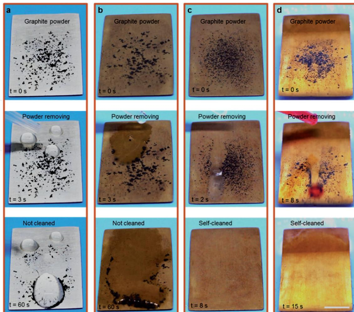
**Figure 1.** Self-cleaning tests on AZ31B Mg alloy. (a, b) time-sequence images showing pristine AZ31B Mg alloy and MnO<sub>2</sub> coated AZ31B Mg alloy surface without self-cleaning properties, time-sequence images showing self-cleaning properties on superhydrophobic surface (c) in air and (d) in oil (isooctane). Scale bar, 1 cm. Reproduced with permission [22]. Copyright 2011, Elsevier.
