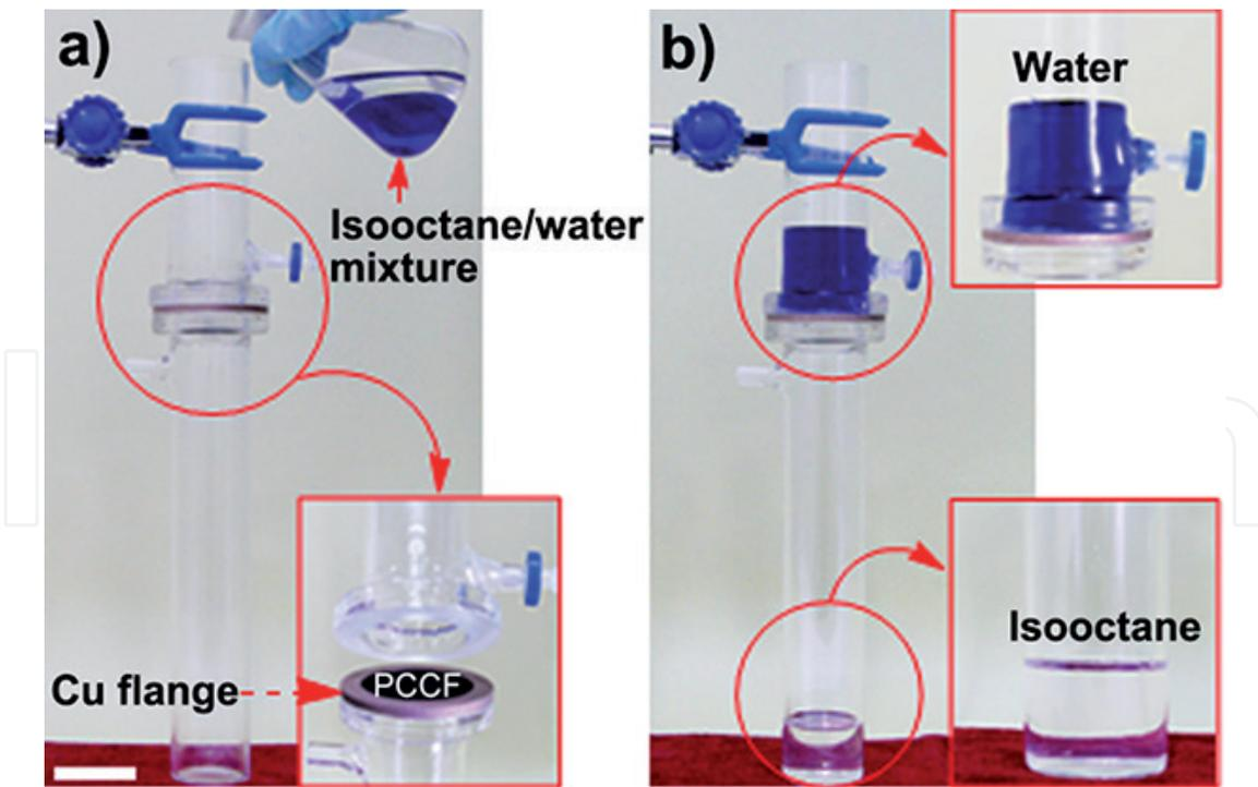
**Figure 2.** Separation apparatus with an 18:25 v:v isooctane/water mixture above PCCF. Inset, PCCF was fixed in Cu flange and then sandwiched between two glass tubes (a). Isooctane passed through PCCF whereas water was retained (b). Water is dyed blue. Scale bar, 3 cm. Reproduced with permission [69]. Copyright 2013, Royal Society of Chemistry.
