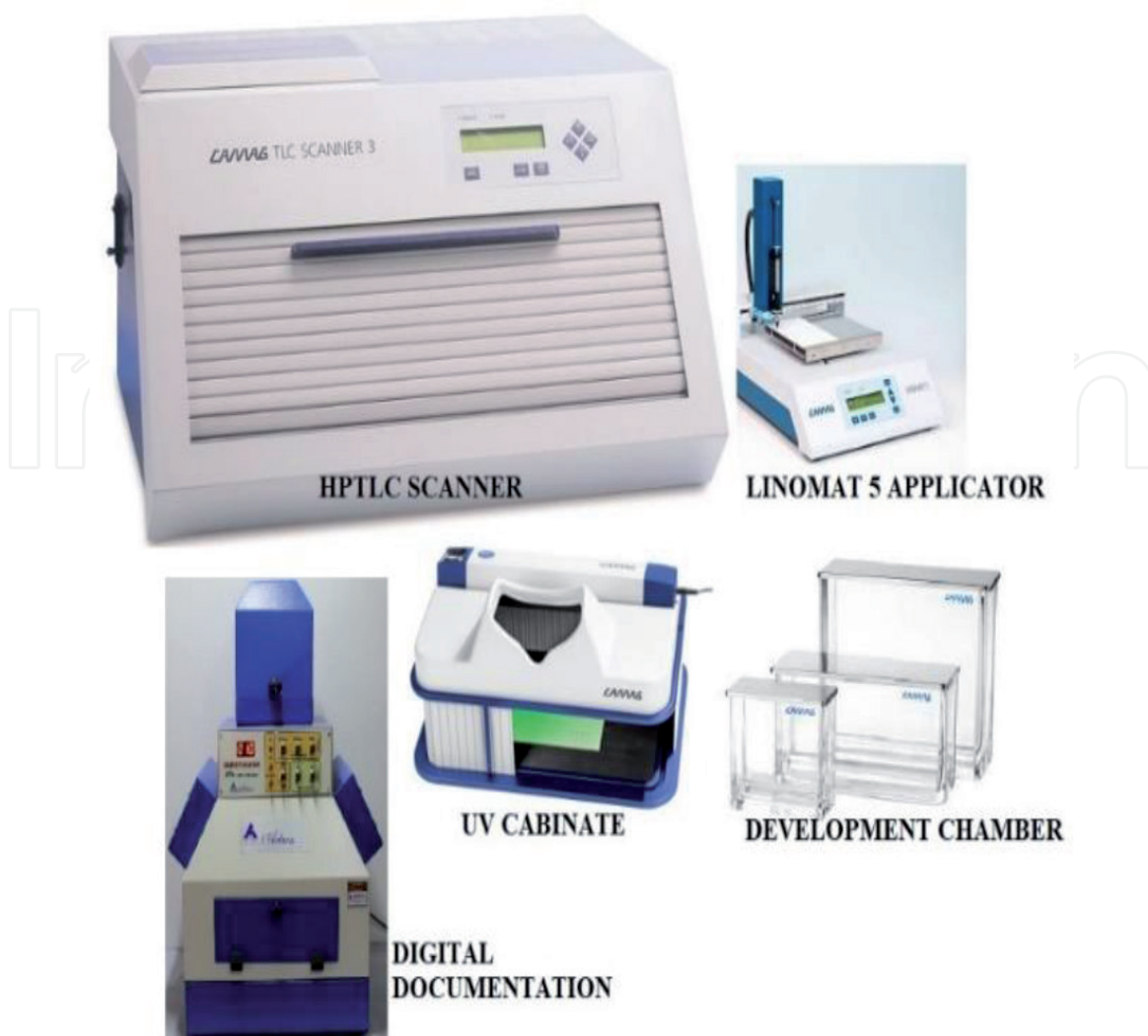
Figure 5. Diagram showing components of HPTLC.
