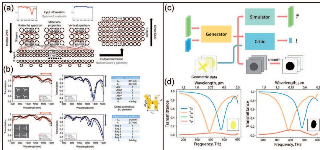
**Figure 3.** Application of DL for plasmonic metasurfaces inverse design: (a) architecture of the DNN composed of xxx. (b) Demonstration of the inverse design of “H”-shaped gold metasurfaces. (c) The architecture of a proposed GAN model composed of a generator, a simulator, and a critic. (d) Transmission spectra of the original (left) and generated (right) patterns from the proposed GAN approach.
