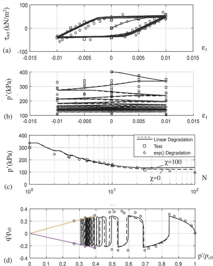
**Figure 1.** Two-way strain-controlled undrained triaxial test simulation of kaolin clay as compared with [2] Grenoble workshop tests and [3]. (a) Shear stress–axial strain relationship. (b) Decreasing mean effective stress with axial strain of  $\epsilon_1 = \pm 1\%$ . (c) Mean effective stress variation. (d) Stress path.
