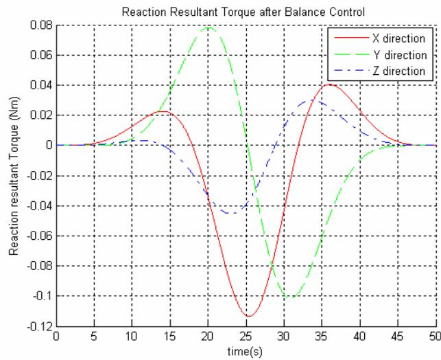
Fig. 4. Reaction resultant torque after balance control.
