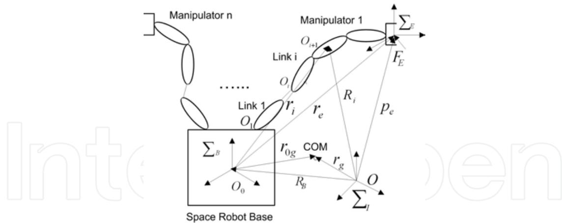
Fig. 1. Dynamics Model of Space Robot System.
