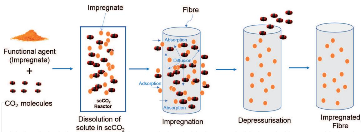
**Figure 1.** Schematic of impregnation mechanism of polymeric fibres with functional agent in scCO<sub>2</sub>.
