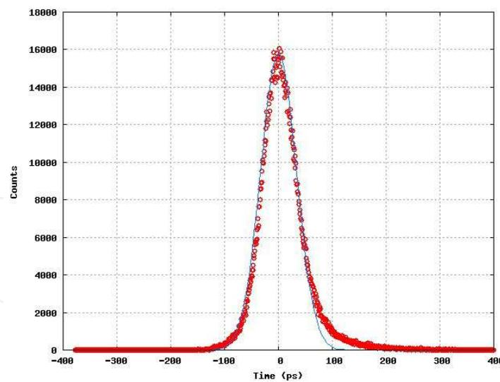
Fig. 14. Time response of silicon photomultiplier (o - experimental measurements, solid line - fit).
