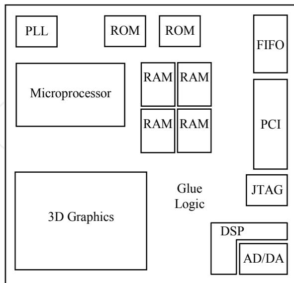
Fig. 1. Structure of core-based system on a chip
