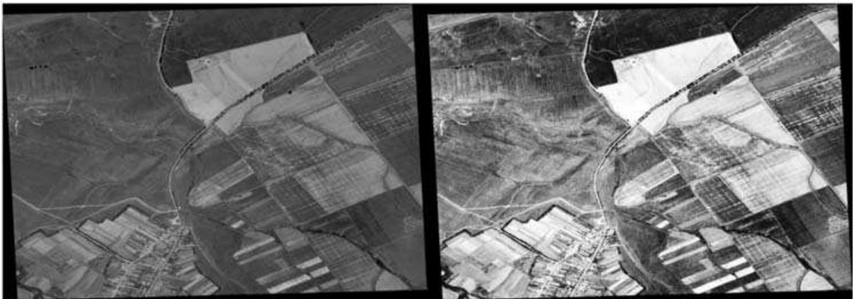
Fig. 3. Histogram equalization: input parameter – an image file; output – the transformed image
