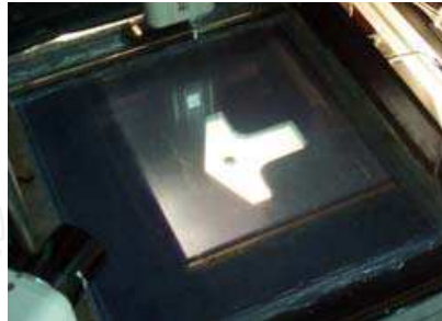
Fig. 3. The LCD photomask of the proposed system
