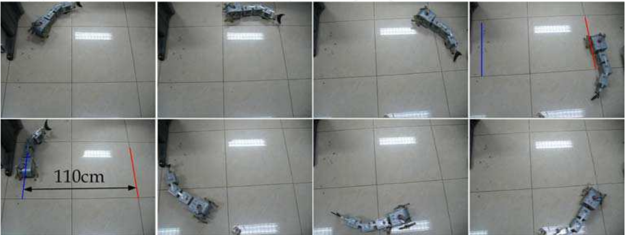
Fig. 14. Image sequence (anticlockwise) of performing circular motion via the body-deformation steering
