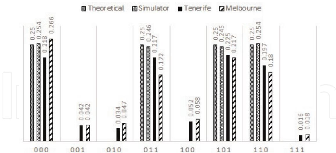
**Figure 3.** Theoretical and experimental implementation of the XOR representation problem on the QASM simulator, Tenerife and Melbourne devices, with 8192 shots.
