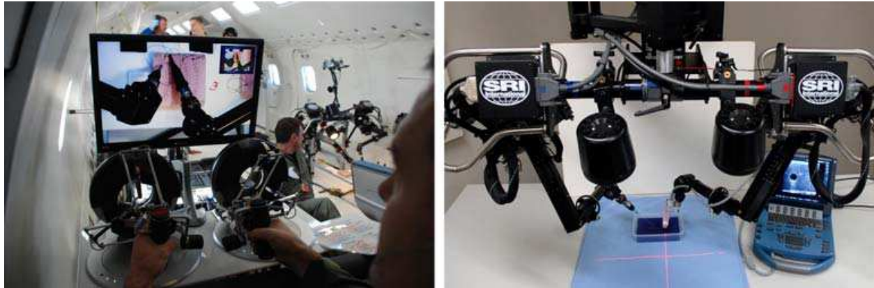
Fig. 7. The M7 on board of a NASA parabolic flight, and the robot performing autonomous ultrasound-guided tissue biopsy. (Photo: NASA, SRI)
