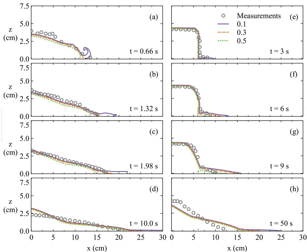
**Figure 5.** The simulated collapsing processes for the initially loose condition (a)–(d) and the initially dense condition (e)–(h). The lines represent contours of the computed concentrations, and the symbols were experimental data of Rondon et al. [40]. The figure is adapted from Lee and Huang [35].
