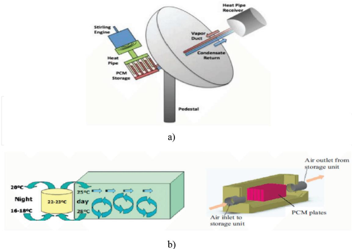
**Figure 1.** NEPCM for energy storage units [1, 2]. a) Latent energy storage for dish striling power generation b) PCM in free cooling systems.
