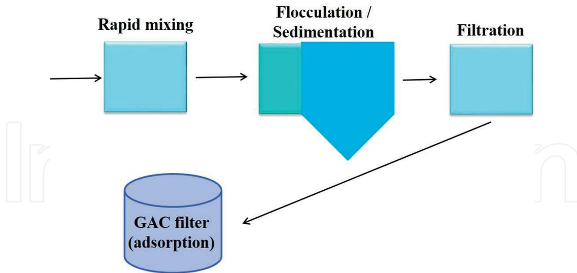
**Figure 1.** Post-filtration process for water purification using GAC.
