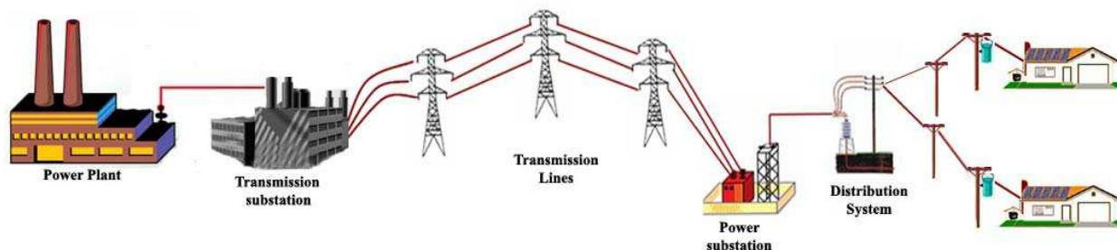
Fig. 1. An example of an electric power system.
