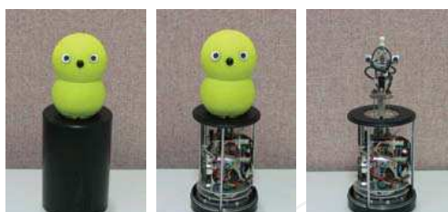
Fig. 4. Keepon’s simple appearance (left) and internal structure (middle/right).
