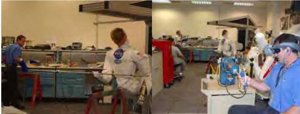
Figure 6. Robonaut working with a human (left) and human teleoperating Robonaut (right) (Glassmire, O'Malley et al. 2004)
