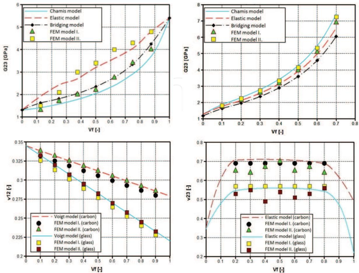
**Figure 10.** Dependence of modulus  $G_{23}$  (left above),  $\nu_{12}$  (left below),  $\nu_{23}$  (right) on  $V_f$  of transversally isotropic composites with epoxy matrix and carbon fibers and glass fibers.
