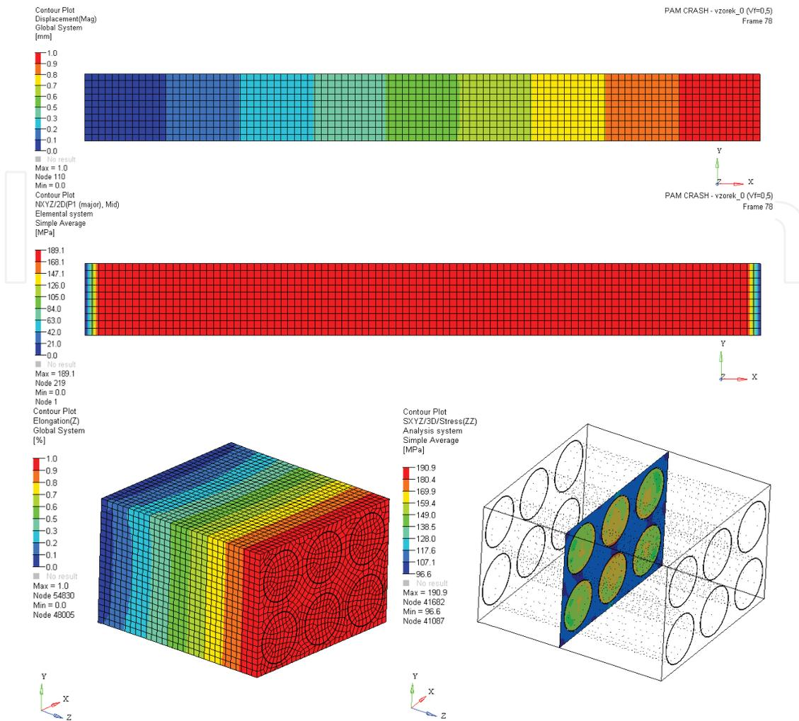
**Figure 12.** Distribution of deformation (above) and principal stress in the loading direction (center) of the FEM model I of long fiber-reinforced composite with epoxy matrix. The resulting distribution of axial strain (below left) and the principal stress acting in the loading direction (below right) and the FEM model II of composite reinforced with long carbon fiber with epoxy matrix.
