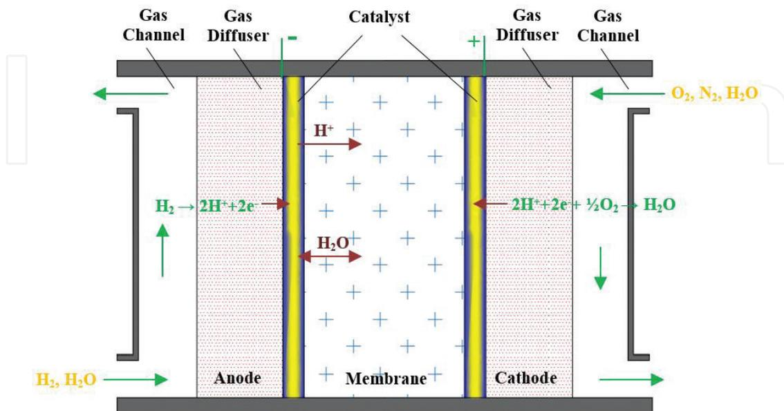
**Figure 1.** A general schematic drawn of PEMFC [1, 2].
